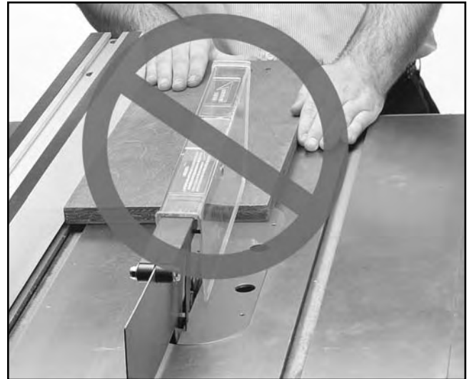
Figure 37. Do not stand directly behind wood.
